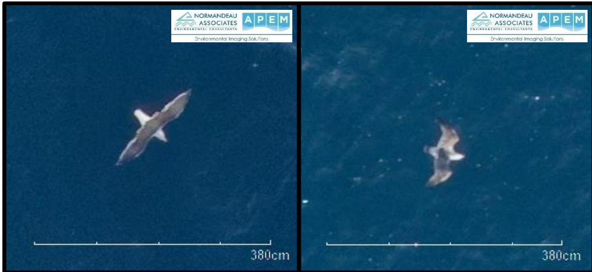
Plate 9 Flying great black-backed gulls of different ages captured in digital still imagery (GSD 1.5 cm)
